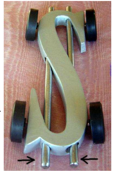
Figure 9. As you can see the metal posts would protrude past the starting post.
