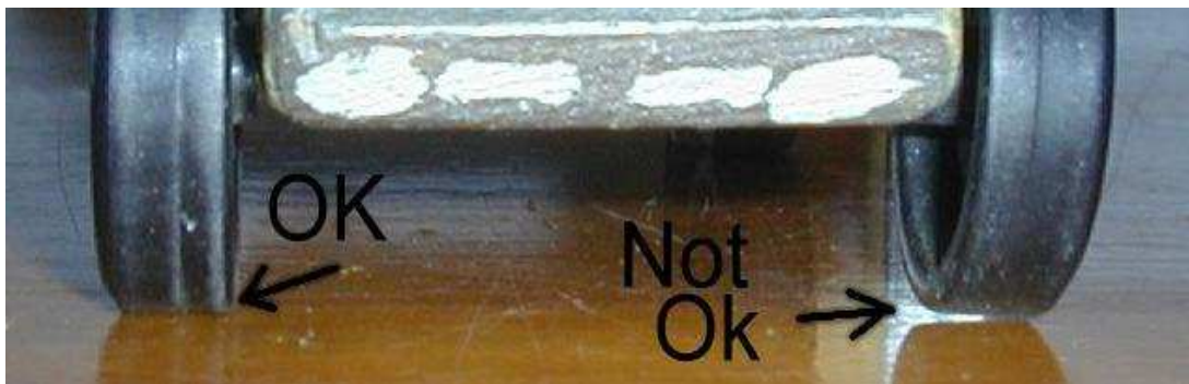
Figure 6. The left wheel is flat to the riding surface, the right is not and would need to be fixed before racing would be permitted
